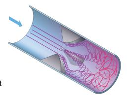
The vane angle, which along with the vortex pairs close proximity to each other, causes the vortices to quickly migrate away from center and towards the pipe wall. The vortices then attach to the pipe wall where they quickly decrease in intensity due to high shear stress at the pipe wall. Rotational momentum is lost. Excessive turbulence is dissipated.
